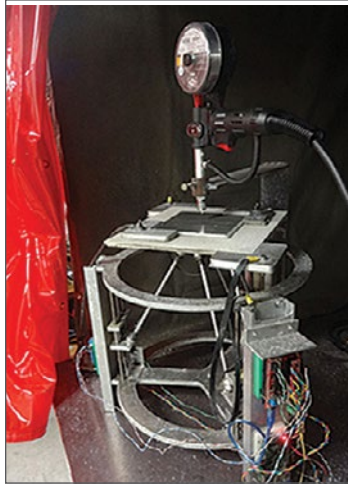
MOST's Magneto 3D printer. Photo by J.M. Pearce. GNU Free Documentation License v 1.3.
